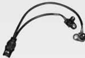
T42436LB EARLY KM PULSE GENERATOR Fits: 96-02 A4AF1/F2, A4BF1/F2, F4A32
