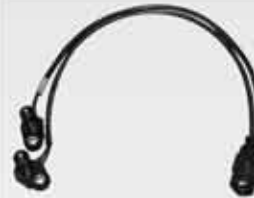
T42436M EARLY KM PULSE GENERATOR Fits: 95-98 F4A33, W4A33
