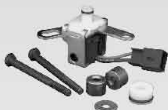
96951U AXOD/AXODE LOCK-UP Fits 86-90 AXOD, 91 Only Taurus Only AXODE 21-36 Ohms, OEM Plug Compatible
