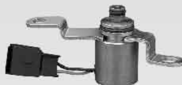
96952 AODE/ AX4S/ AX4N EARLY MCCC Fits 91-94 AODE, 93-97 AX4S, 95-96 AX4N .98-1.6 Ohms, OEM Plug Compatible
