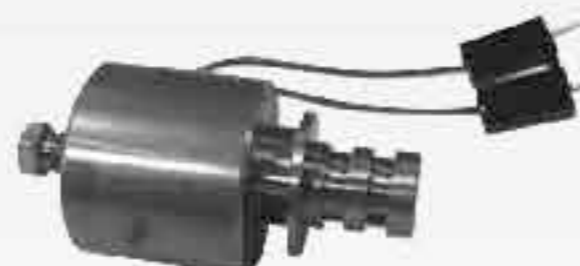
82840 ZFHP22 EPC Fits 84-94 ZF4HP22, 88-94 ZF4HP24 3.5-4.66 Ohms, NOTE: 5 Solenoid Valve Body ONLY!!
